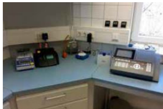
Fig. 3: photoLab® 7600 UV-VIS photometer for the measurement of optical, reagent-free (OptRF) methods in the laboratory of the WWTP Peißenberg
